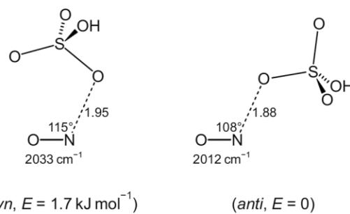
**Figure 5.** The two minima of about equal stability on the conformational hypersurface of an NO(HSO<sub>4</sub>) entity on the BP86/def2-TZVP level of theory (N–O distances in Å), and the corresponding N–O stretches; compare:  $\nu$ (NO) = 2358 cm<sup>−1</sup> for the free NO<sup>+</sup> ion calculated on the same level.
