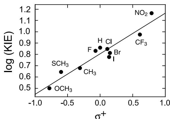
Fig. 5. Substituent dependence of the deuterium kinetic isotope effect for benzyl alcohol oxidation. Semi-log plot of observed  $k_{\text{H}}/k_{\text{D}}$  rate ratio versus the electronic substituent parameter Hammett  $\sigma^+$  for a series of *para*-substituted benzyl alcohol derivatives.
