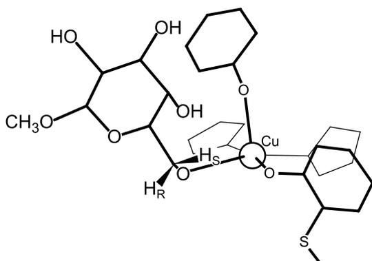
Fig. 3. Model for substrate complex with galactose oxidase. The orientation of the substrate is constrained by steric interference with Phe194, Trp290, Phe464, and Arg330. Prochiral hydrogens of the substrate  $\alpha$ -methylene group are labeled.
