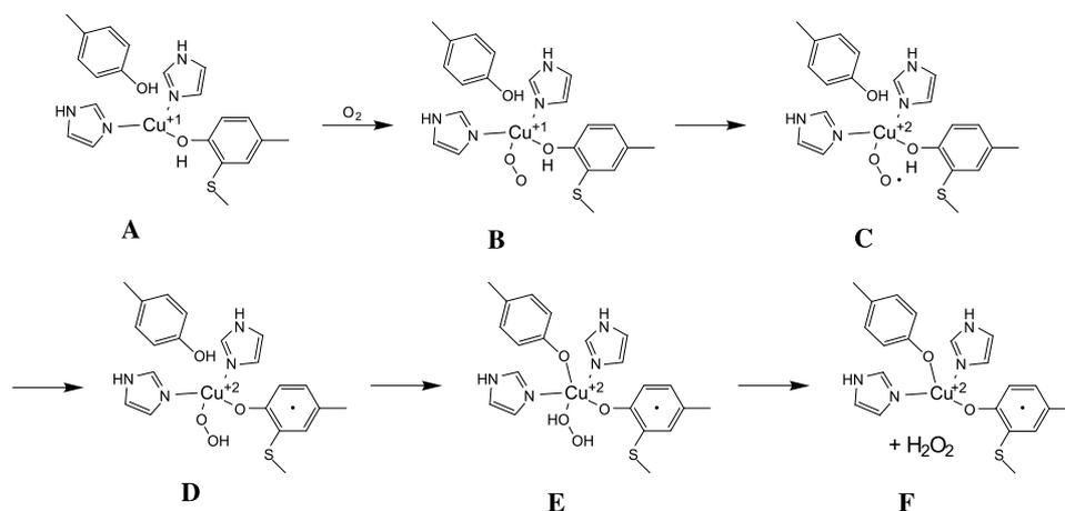
Fig. 6. Proposed mechanism for dioxygen reduction by galactose oxidase. Reaction of  $O_2$  with the  $Cu^{I+}$  active site (A) is predicted to involve formation of an adduct (B) that will undergo single-electron transfer to form an oxy radical complex (C). Hydrogen abstraction reduces the complex to a hydroperoxide adduct (D) which may be protonated at the proximal oxygen (E) leading to displacement of the product (F).
