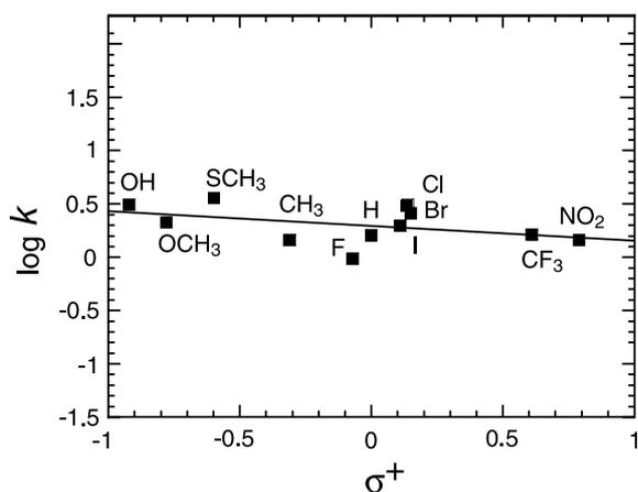
Fig. 4. QSAR analysis of the galactose oxidase turnover reaction. Rate data for enzymatic oxidation of a series of *para*-substituted benzyl alcohols is plotted versus the electronic substituent parameter Hammett  $\sigma^+$ . The correlation slope is  $\rho = -0.09 \pm 0.32$ .
