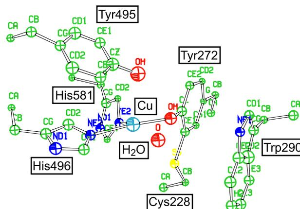
Fig. 1. The active site of galactose oxidase. The active site metal ion (Cu), inner coordination sphere (Tyr272, Tyr495, His496, His581, and coordinated solvent) and Trp 290 in the outer sphere of the complex. Based on PDB ID 1gog. Rendered using ORTEP-III [36].
