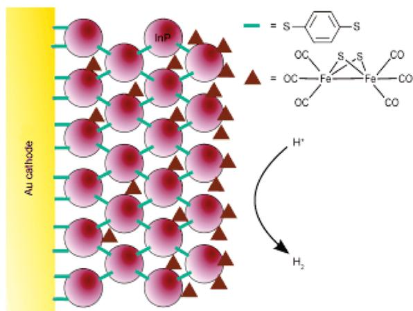
**Figure 8.** Cross-section of a InP nanocrystal modified gold electrode with adsorbed/intercalated  $\text{Fe}_2(\text{S}_2)(\text{CO})_6$  subsite analogue. Reproduced with permission from ref 156; copyright Wiley-VCH Verlag GmbH & Co. KGaA.
