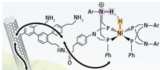
**Figure 7.** Ni complex attached to multiwalled carbon nanotubes in a high-surface area cathode material by Le Goff, from the Perspective by Hambourger et al. in ref 149. Reprinted with permission from the AAAS.
