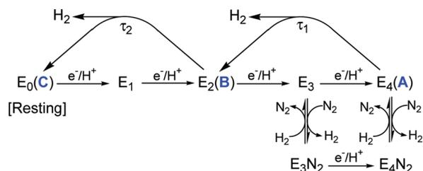
**FIGURE 1.** Early stages of Lowe–Thorneley (LT) kinetic scheme for  $N_2$  reduction, the portion that connects states  $E_0$  through  $E_4$ ; for a full scheme, see refs 2–4. As discussed in conjunction with Figure 8, **A** is the MoFe protein “hydride” intermediate; **B** forms during its relaxation to resting state, **C**.
