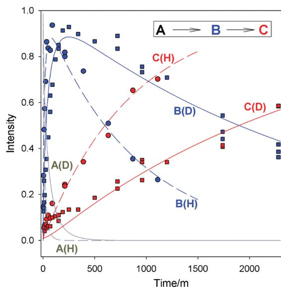
**FIGURE 8.** Step-annealing curves (253 K) of hydride intermediate (**A**), leading to formation of **B** intermediate and ground state **C**, in  $H_2O/D_2O$  buffers. Fits to distributed (stretched exponential) two-step relaxation:  $t_1(H_2O) = 13$  min,  $t_1(D_2O) = 49$  min;  $t_2(H_2O) = 870$  min,  $t_2(D_2O) = 2700$  min. For clarity, data for **A(H)** and **A(D)** are omitted, and only the fits are presented.
