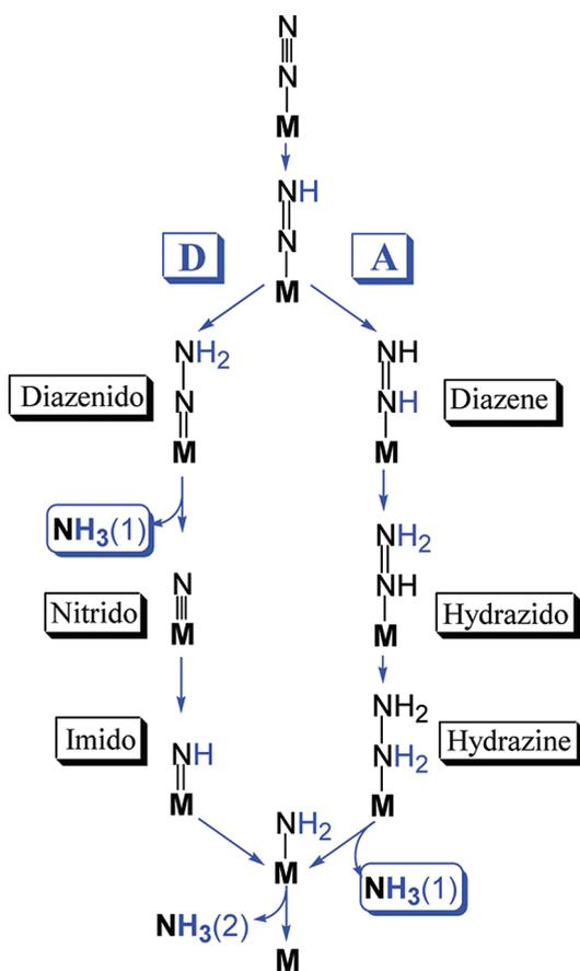
**FIGURE 4.** “Alternating” (A) and “distal” (D) N<sub>2</sub> reduction pathways. M represents FeMo-co without specifying metal ion(s) involved. Likewise, the representations of binding are meant to emphasize the distinction between pathways and do not imply specific binding modes. Small straight arrows represent addition of H<sup>+</sup>/e<sup>-</sup> to substrate.
