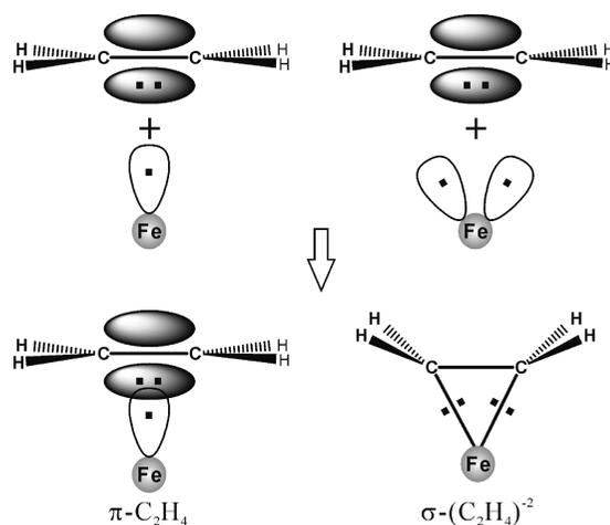
**FIGURE 6.** Cartoon representation of alternate schemes for binding C<sub>2</sub>H<sub>4</sub> to a cofactor metal ion: (left) dative  $\pi$  bonding; (right) oxidative addition to form Fe–C  $\sigma$  bonds.
