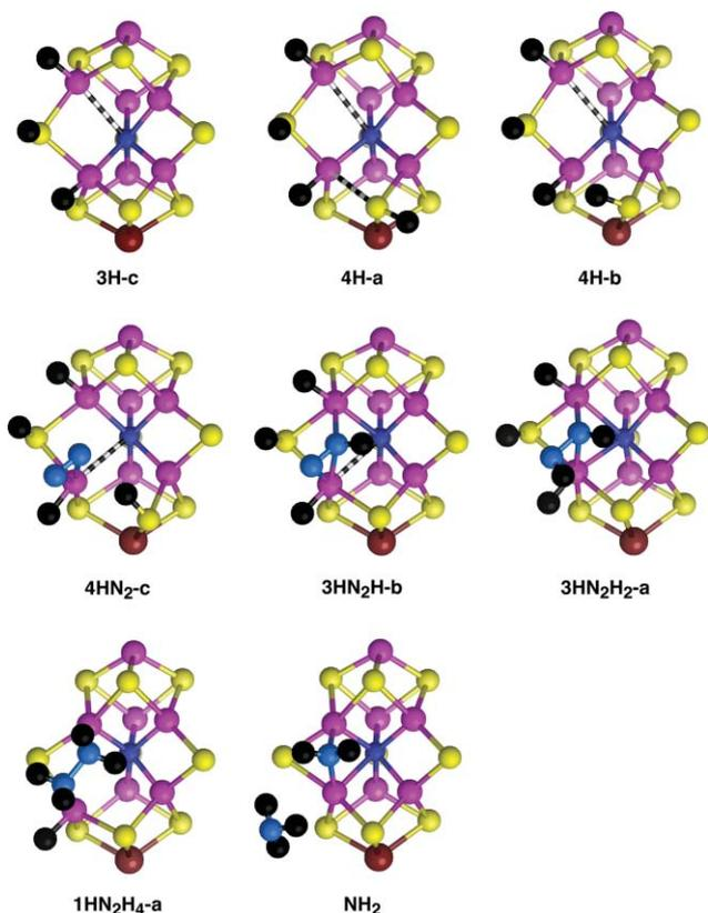
**Fig. 4** Optimised structures of some key intermediates in the proposed mechanism (cf Fig. 3). The view direction is perpendicular to the Fe<sub>2</sub>,Fe<sub>3</sub>,Fe<sub>6</sub>,Fe<sub>7</sub> face (similar to Fig. 1). Fe magenta, S yellow, Mo brown, N blue, H black: the terminal ligands bound to Fe<sub>1</sub> and Mo are not shown. N<sup>c</sup>-Fe and Fe-S distances in the range 2.5-3 Å are marked as black and white broken bonds.
