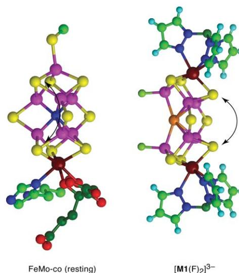
**Fig. 5** Comparative side views of FeMo-co (structure PDB 1M1N) and  $[\text{M1}(\text{F})_2]^{3-}$  (structure CSD VEGCAM,  $\text{S}^c$  orange) to show the relative opening of the rear  $\text{HS-Fe}(\mu_6\text{-S})\text{-Fe-SH}$  section and concomitant closing of  $(\mu_3\text{-S}) \cdots (\mu_3\text{-S})$  (arrowed) on the front  $\text{Fe}_4\text{S}_4$  face.
