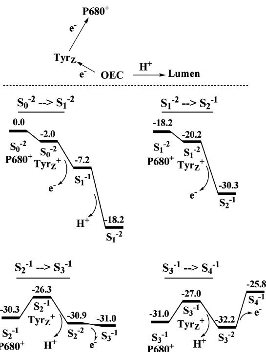
FIGURE 9. Energy diagrams for the different S-transitions, including Tyr<sub>Z</sub> oxidation.
