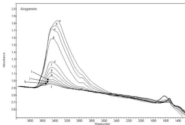
**FIGURE 8.** Temperature-resolved IR spectra show a decrease in the intensities of the OH bands in the region of 3000–3600 wave numbers starting at ~200 °C. (a) 26 °C, (b) 100 °C, (c) 150 °C, (d) 200 °C, (e) 250 °C, (f) 260 °C, (g) 270 °C, (h) 280 °C, (i) 290 °C, (j) 300 °C, (k) 310 °C, and (l) 320 °C.
