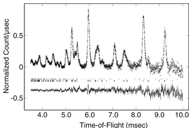
**FIGURE 2.** Final observed (crosses), calculated (solid line), and difference (lower) powder diffraction patterns for the Rietveld refinement using the neutron powder diffraction data. The background has been subtracted and the intensities have been normalized to the incident spectrum.
