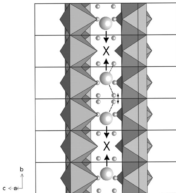
**FIGURE 5.** Schematic drawing showing a possible Cl anion ordering scheme in the akaganéite tunnels. The small circles represent the H atoms, and the larger circles in the tunnel region indicate Cl anions. Vacant tunnel sites are indicated by "X".
