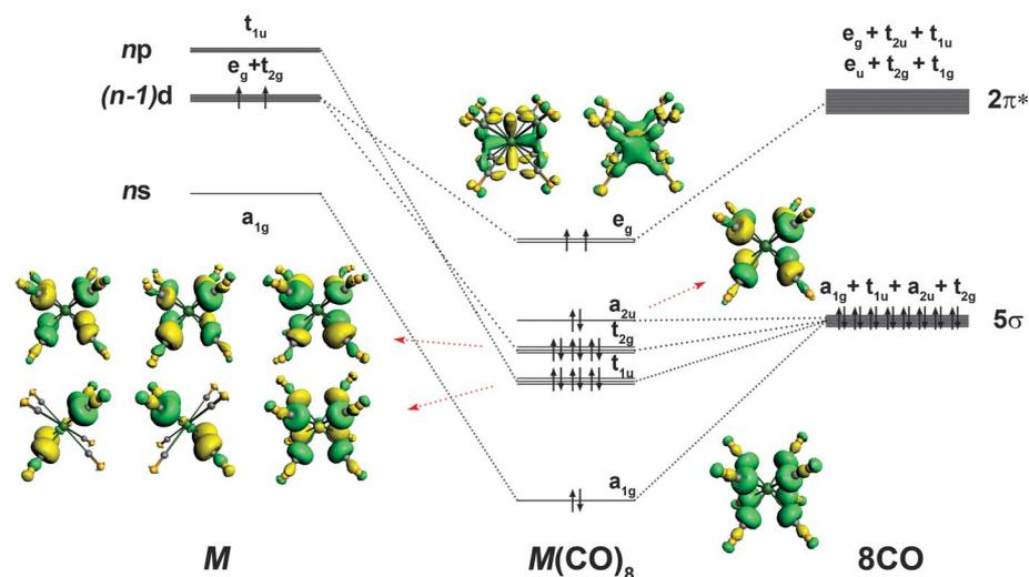
**Fig. 3. Bonding scheme and shape of the occupied valence orbitals of  $\text{M}(\text{CO})_8$  (M = Ca, Sr, or Ba).** Splitting of the spd valence orbitals of an atom M with the configuration  $(n-1)d^2ns^0np^0$  in the octacoordinate cubic ( $O_h$ ) field of eight CO ligands is also given. Only the occupied valence orbitals that are relevant for the M-CO interactions are shown. Up and down arrows indicate electrons with opposite spin.
