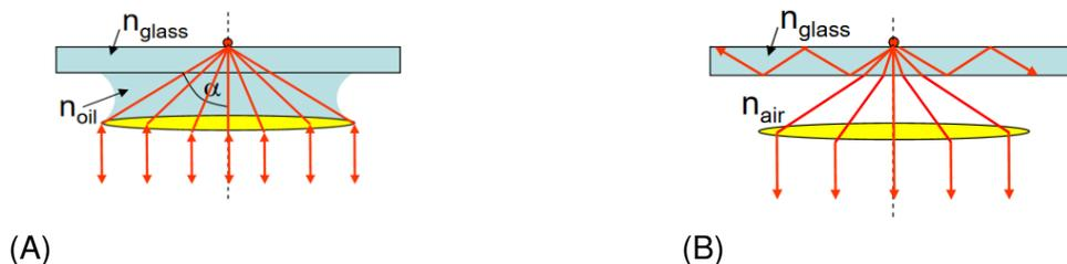
**Figure 12:** Illustrations of the beam path in (A) the case that the refractive indexes of glass and immersion medium are the same and in (B) that the reflection index is smaller than the one from glass, for example air(1.0).<sup>[51]</sup>
